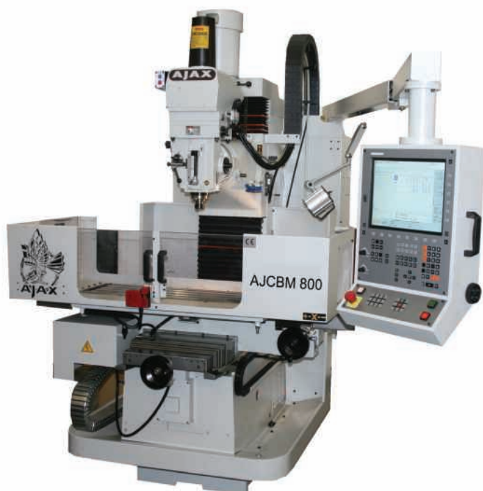
Ajax's AJCBM 800 is the first UK built machine to feature the latest version of Heidenhain's popular TNC 320 control
