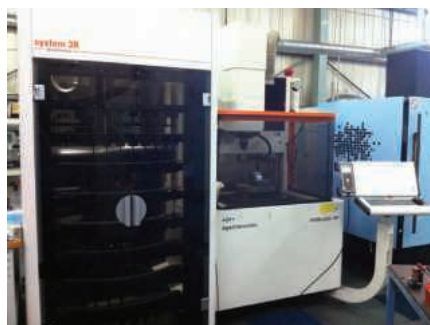
The System 3R WorkPartner robot working alongside the AgieCharmilles Form 2000 HP spark erosion machine
