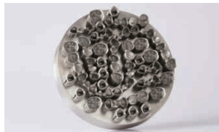
Approximately 70 dental crowns and bridges made from EOS CobaltChrome SP2 in three hours in an EOS M 100 system
