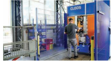
The two-station design allows for simultaneous welding and loading of the compact cell
