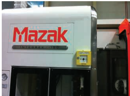
Emergency manual release switch on a Mazak machine
