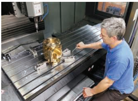
Ian Cocker removing a bronze ball valve after finish machining on the VMX84SWi
