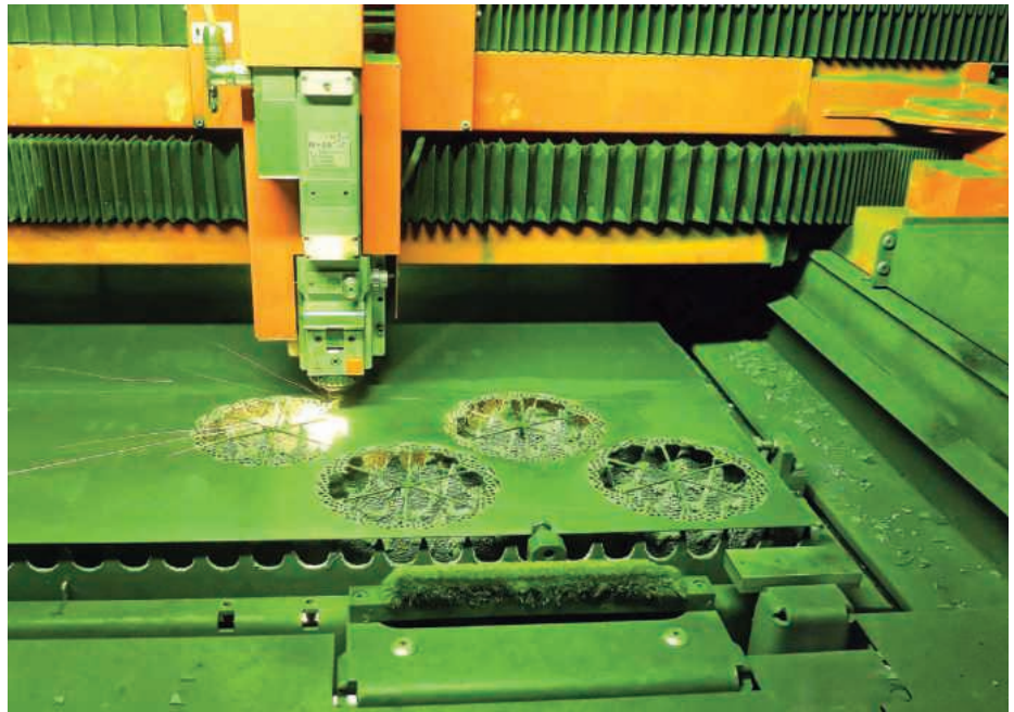
Brake discs being machined from 410 stainless steel on the BySprint Fiber 3015 at Hope Technologies (photographed through a green-tinted glass window that absorbs reflected, short-wavelength laser rays to protect the operator's eyes)
