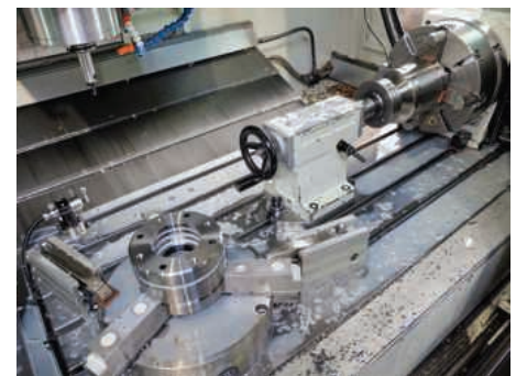
Two components are fixed on the table of the VMX50, one in a 4th axis and tailstock arrangement. Both are condition H900 17-4 PH stainless steel components for an oil industry development project
