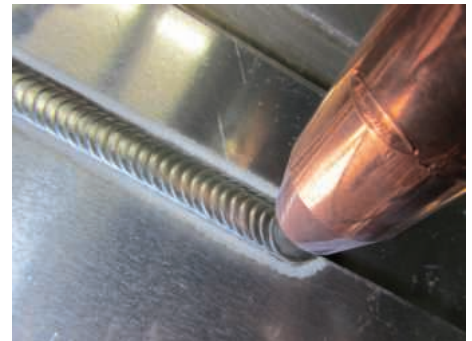
An optimally weaved and spatter-free weld seam produced in aluminium using PMC mix drive is visually indistinguishable from a TIG seam
