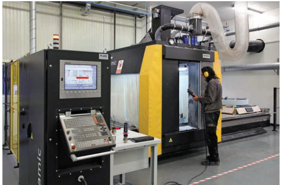
The Blue Ray Sahos Dynamic FC5000 5-axis machining centre at Lentus Composites produces mainly one-off patterns, composite components and aluminium moulds
