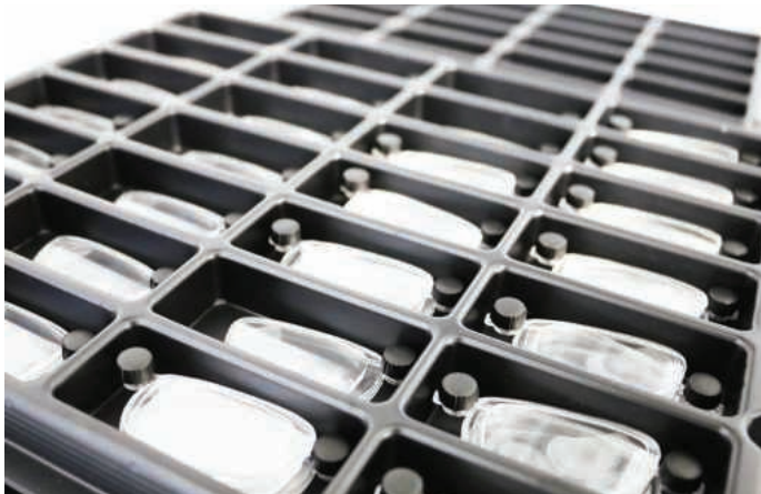
The finished and assembled product is placed into a thermoformed tray by one of the robots in the production cell
