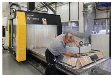
Lentus production manager Rupert Truman inspecting a superconducting magnet coil after OD milling in the Sahos Dynamic
