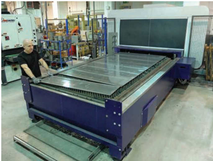
Stainless steel is supplied to Hope in various sizes. Here, eight sheets measuring 1,500 mm x 375 mm are being laid across the shuttle table of the BySprint Fiber 3015
