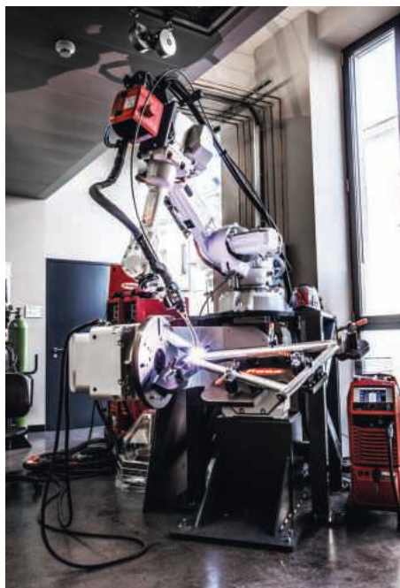
A realistic test setup has clearly shown that PMC mix drive can be used to weld up at speeds of up to 30 cm per minute in aluminium and is therefore considerably more cost-effective than ever before
