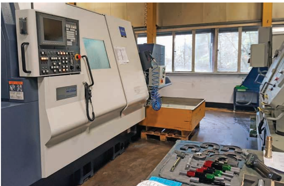
The Bar turn-mill centre Miyano BNE-51 MSY installed at MCS in Redditch
