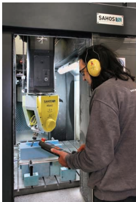
The machining area of the Sahos Dynamic, showing the A-surface of a pattern for an F1 component being machined from epoxy tool board
