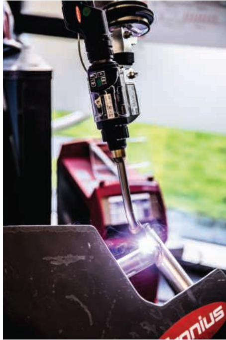
PMC mix drive harnesses the possibilities offered by a powerful PullMig welding torch, such as the Robacta Drive, to control the heat input even more precisely when welding aluminium, CrNi or vertical-up seams in steel
