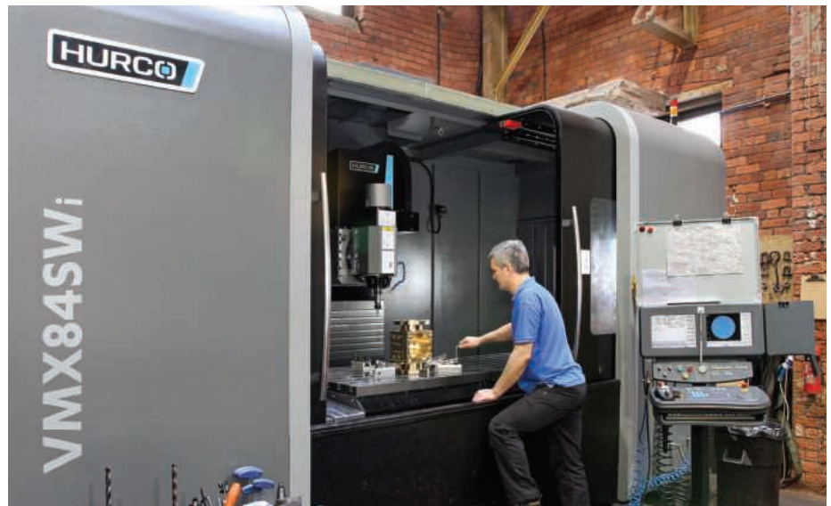
The Hurco VMX84SWi machining centre at Ian Cocker Engineering's Sheffield factory has a 12,000 rpm/22 kW, swiveling B-axis spindle, through-spindle coolant and 40-station tool magazine
