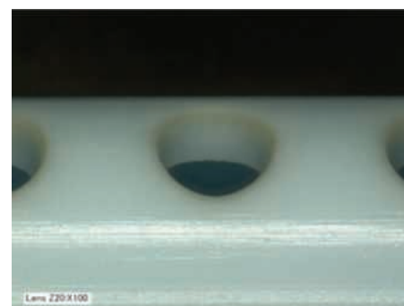
Comparison of 1030 nm fs disk laser to a 355 nm ns laser when drilling polypropylene
