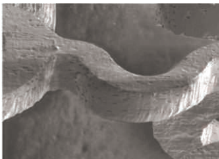
Figure 3 shows the high cutting quality of the fs laser for cutting of Nitinol stent
