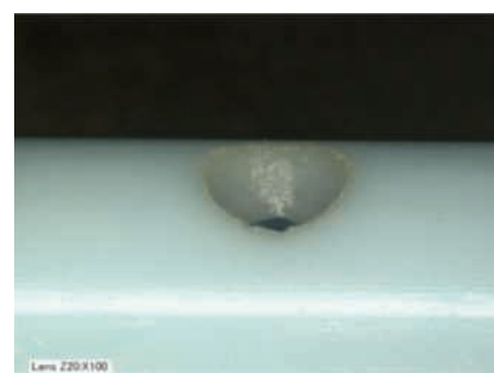
Comparison of 1030 nm fs disk laser to a 355 nm ns laser when drilling polypropylene
