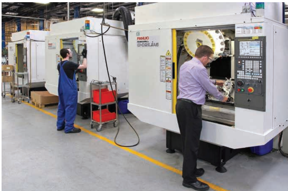
The line of three Fanuc \alpha -D21LiA5 Robodrills in the new oil and transmission pump manufacturing cell at Concentric's factory in Erdington, Birmingham
