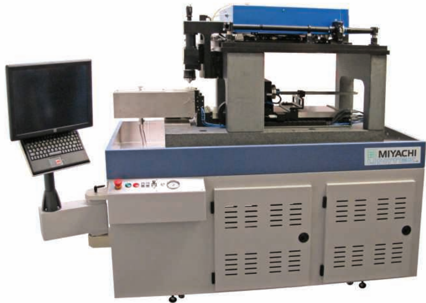
Femtosecond stent and hypo tube cutter, covers off, showing Jenoptik laser
