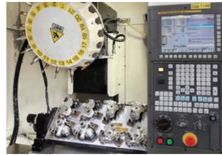
The third Robodrill is devoted to producing two pairs of transmission pump components per cycle
