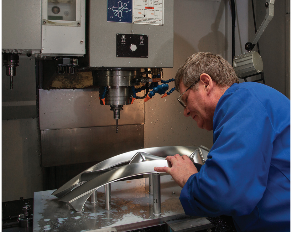
Talon's Process Engineer Sandy Bradley inspects the result of almost one million lines of NC code
