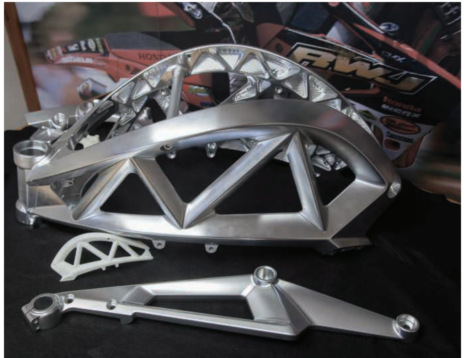
The left hand 'Wing Spar' frame member of the Ariel Ace motorcycle. The machined finish was a specification of Ariel
