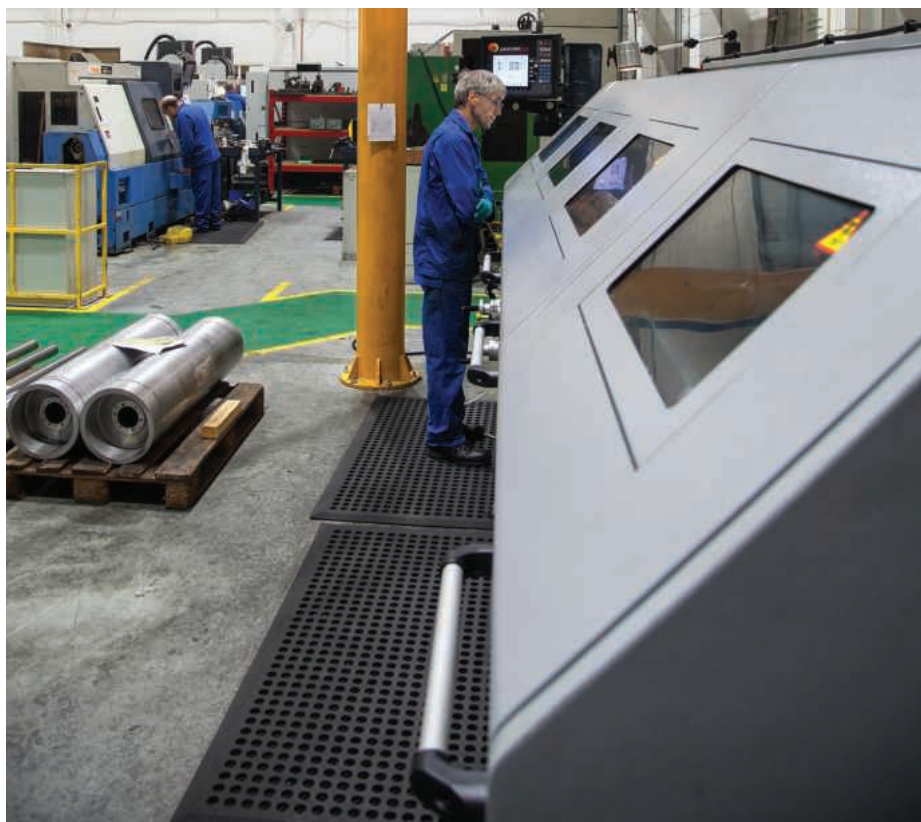
Above and Below: The XYZ SLX 555 ProTURN lathe is used on a wide variety of components from gears to large rollers, replacing capacity left after a high value turning centre was removed
