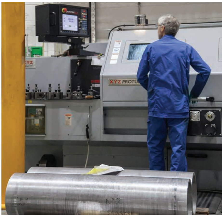
Above and Below: The XYZ SLX 555 ProTURN lathe is used on a wide variety of components from gears to large rollers, replacing capacity left after a high value turning centre was removed
