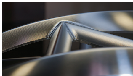
The machined surface on the external face was specified by Ariel. On the inside face, deep pockets remove even more weight from the original 150 kg billet
