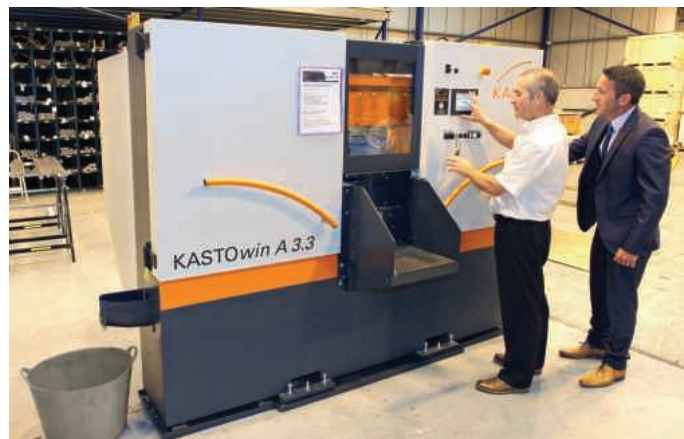
Robin Dawson programming the KASTOwin A 3.3 for cutting the next batch of alloy billets
