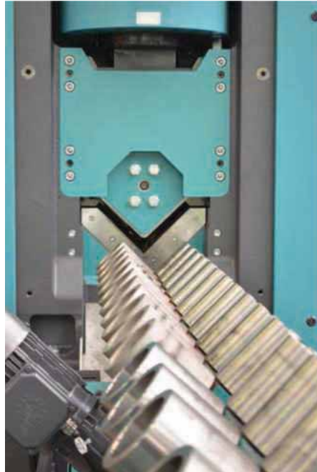
Automatic measurement of the legs or material thickness minimises operator errors and achieves optimal tool positioning
