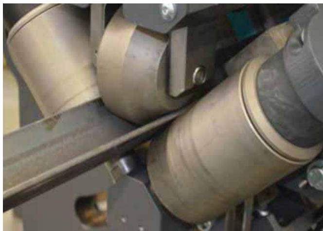
Automatic measurement of the legs or material thickness minimises operator errors and achieves optimal tool positioning
