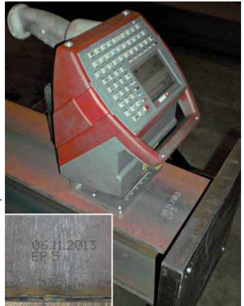
The FlyMarker PRO hand-held marking system in action marking a welding seam
