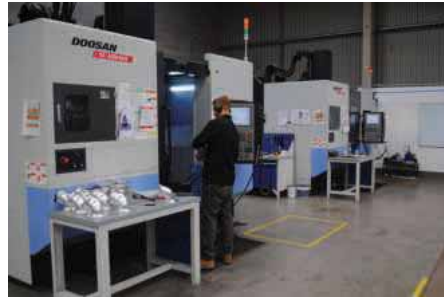
AVPE's 5-axis machining cell showing the 2 x Doosan VC630 5AX 5-axis machines in action
