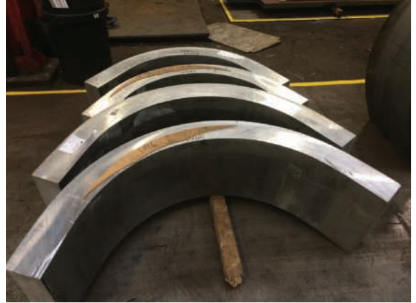
To achieve precision and tight curvature, Barnshaws recommended the use of high quality aluminium 5083 that had been annealed to reduce the risk of cracking
