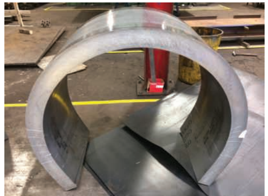
The level of precision required for the curvature of each section was required to hundredths of a degree, with eight different radii specified for the sections ranging from 101.09° to 212.40°
