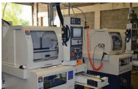
Braintree Precision Components is using Miyano GN-3200 to replace grinding processes with hard turning
