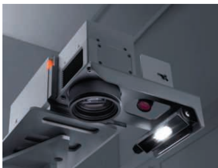
Immediately after the marking process, a camera reads the code generated and marked on the component
