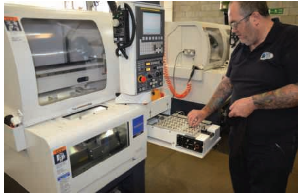
Pallet loading of inner ring bearing components as part of integrated loading and machining sequences at Braintree Precision Components
