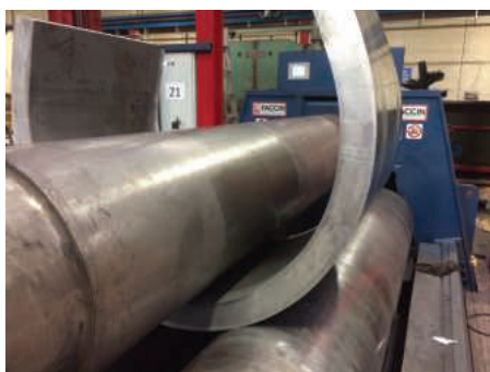
Barnshaws produced ten rolled aluminium sections, up to 800 mm in length and varying in thickness from 83 mm to 114 mm
