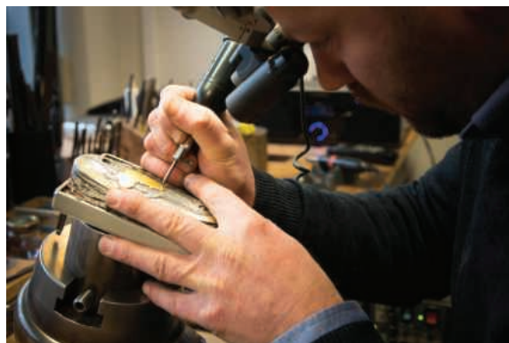
Vince Crowley engraving a prestige gun using a Minimo hand-piece
