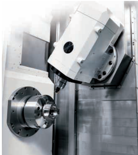
The X-axis on the NTRX 300 has a 125mm travel below the spindle centre to extend the machining range to 250mm square
