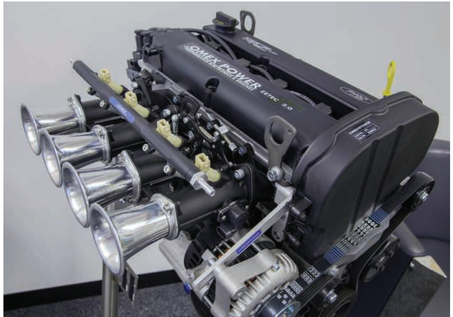
A Zetec engine fitted with Omex's new throttle bodies and fuel injection system, with most parts being machined on the XYZ 1020 VMC
