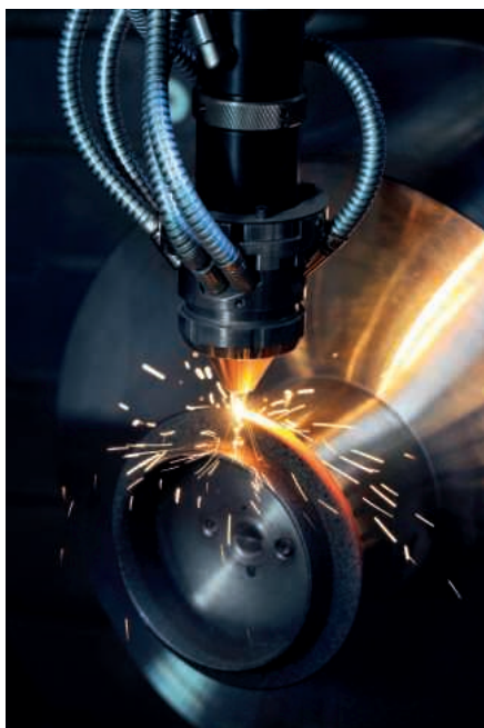
Above and below: Additive manufacturing: DMG MORI combines laser deposition welding and milling in a single setup with the LASERTEC 65 3D
