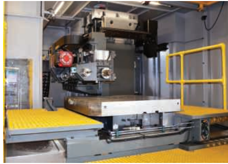
Mollart Prismabore combines gundrilling and conventional machining centre spindles in one machine.
