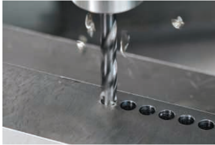
Sumitomo's SumiDrill SDP is designed for holes up to 7xD between 3 and 16 mm diameter
