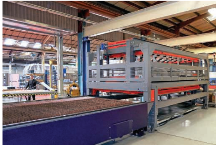
The ByTrans 4020 Extended automated sheet handling system (right) linked to Syspal's BySprint Fiber 4020
