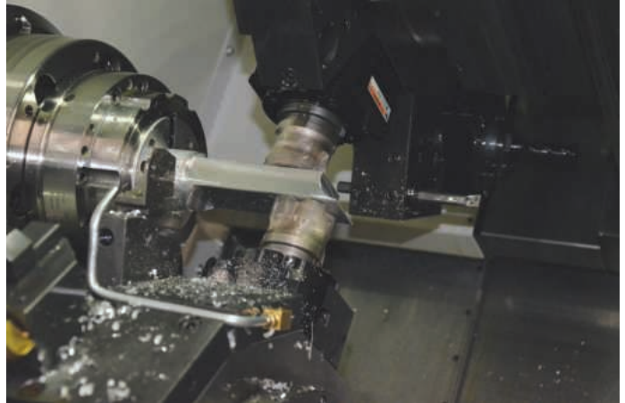
Twin turrets enable opposed head milling on Wealdpark's Miyano ABX-64SYY2 turn-mill centre
