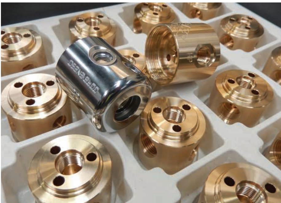
Production savings of almost £4,000 have been made in just eight weeks on both types of port bodies produced in single cycles on the Miyano BNE-51MSY at Apeks Marine Equipment
