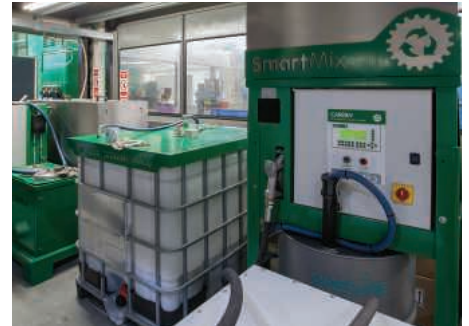
The Cardev Coolant Cleaning System and Smart Mix work in tandem to keep the 18 machines at Proseal supplied with coolant, either recycled or freshly mixed
