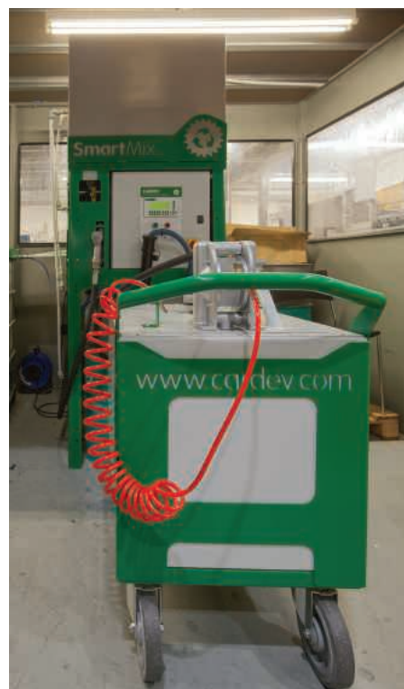
The Cardev Smart Mix system automatically creates fresh metalworking fluid solution to the correct concentration. This can then be supplied directly to the machine via a pipe system or via the Cardev coolant transfer unit
