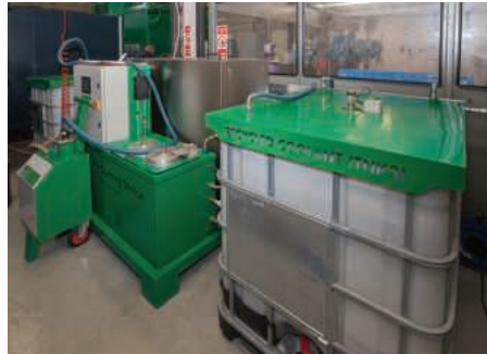
The Cardev Coolant Cleaning System and Smart Mix work in tandem to keep the 18 machines at Proseal supplied with coolant, either recycled or freshly mixed
