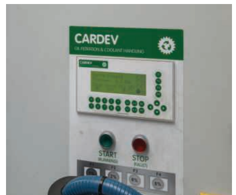
The Cardev Smart Mix system automatically creates fresh metalworking fluid solution to the correct concentration. This can then be supplied directly to the machine via a pipe system or via the Cardev coolant transfer unit
