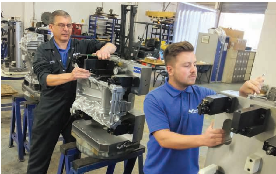
Hydraulic tombstone op10 fixture to suit the horizontal machining centre
