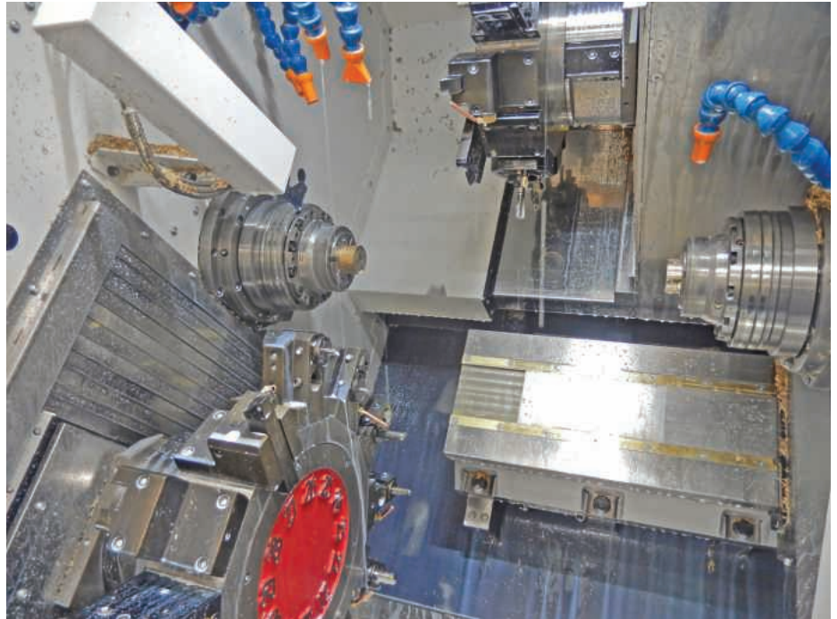
The Miyano BNE-51MSY is tooled to produce safety-critical regulator components at Apeks Marine Equipment
