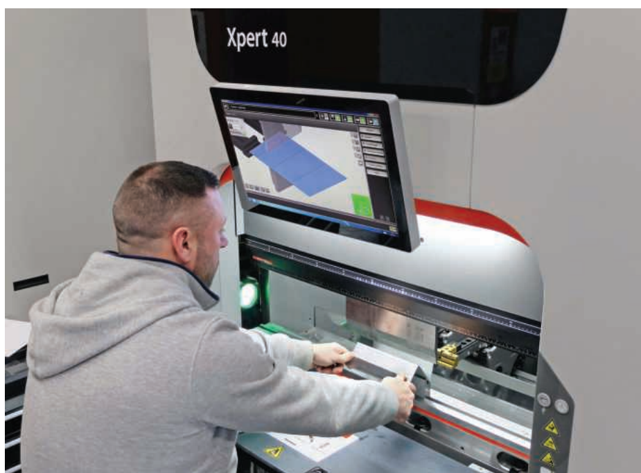
The 40-tonne Xpert press brake is very fast when bending parts up to its maximum capacity of one metre
