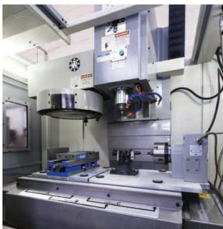
The use of the Jergens Ball Lock system on the XYZ LPM and XYZ 2-OP has brought increased efficiency to Batchflow's milling operations
