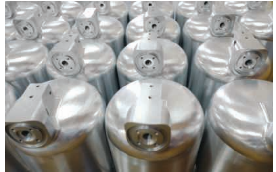
High-precision components machined on Aerotech's new Doosan VCF 850LSR 5-axis machining centre
