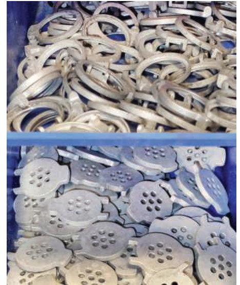
Typical aluminium switch cover components produced by Dicker Precision on the B465-T2Y2. Bases are seen at the top and covers below
