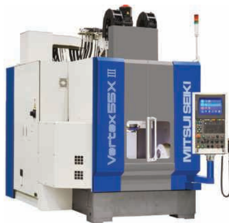
Mitsui Seiki Vertex 55X III from 2D CNC Machinery introduces MAMS multi-sensor thermal growth monitoring to 5-axis machining
