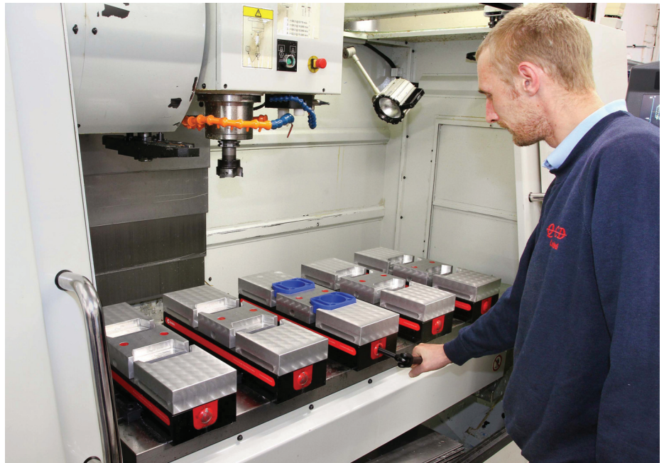
Five Chick Qwik-Lok twin-station workholding units from 1st MTA on the table of a vertical machining centre at Gosport-based subcontractor, QCD
