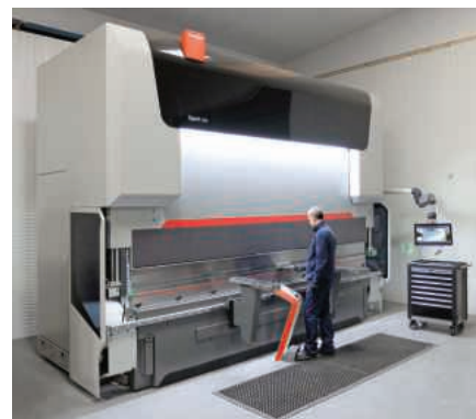
The Xpert 250 press brake, rated at 250 tonnes, is capable of bending parts up to 4.1 metres
