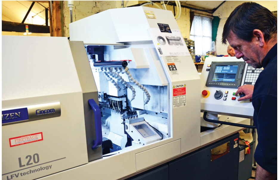
Machine setter Darren Evans maintains the wiper action created using the tool with Citizen's LFV technology producing a superior surface finish
