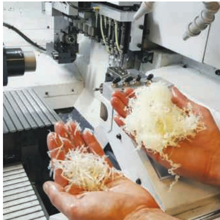
Plastics 'birds-nesting' in the right hand without LFV on the Citizen L20-VIII and the cutting process totally under control with programmed chip lengths using LFV in the left hand
