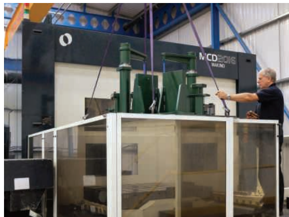
A large fixture being manoeuvred onto the second pallet of the Makino MCD 2016
