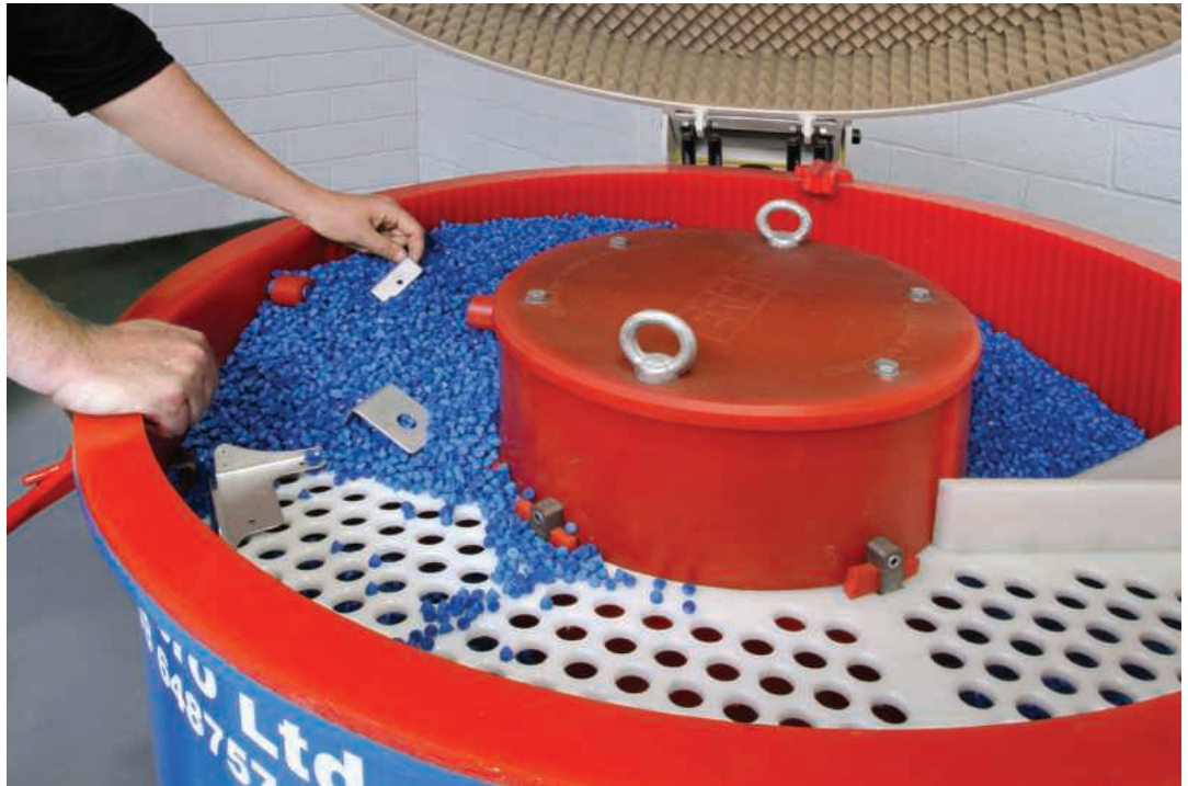
ESP Laser Cutting says that its vibratory finishing bowl from PDJ Vibro stress-relieves the case hardening that occurs around the edges of laser-cut sheet metal components
