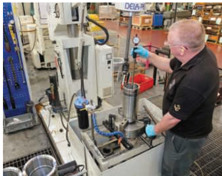
Image 1 and 2: A Kitagawa JN12T manual scroll chuck clamping an Oleo type 4 rail buffer cylinder for machining on a Delapena vertical PowerHone
