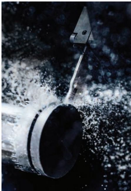
The DirectCooling System delivers optimum working temperature as well as ideal chip evacuation which together ensures the highest level of reliability
