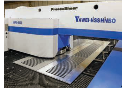
A view from either end of the punch press showing 3 mm thick aluminium sheet being machined for new student residential accommodation at Eastside Locks in Birmingham
