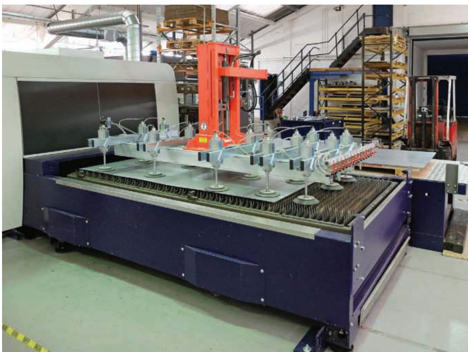
The Byloader at Wheeler Fabrications transferring a new sheet onto the shuttle table of the Bystronic fibre laser cutting machine
