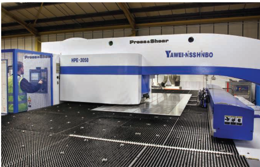
The Yawei-Nisshinbo HPE-3058 turret punch press installed at Weldall's factory in Cannock
