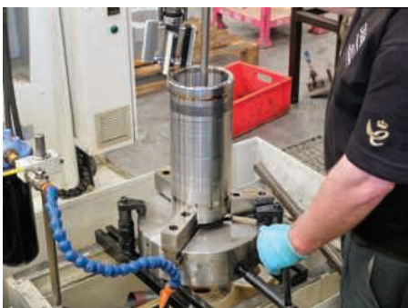
Image 1 and 2: A Kitagawa JN12T manual scroll chuck clamping an Oleo type 4 rail buffer cylinder for machining on a Delapena vertical PowerHone
