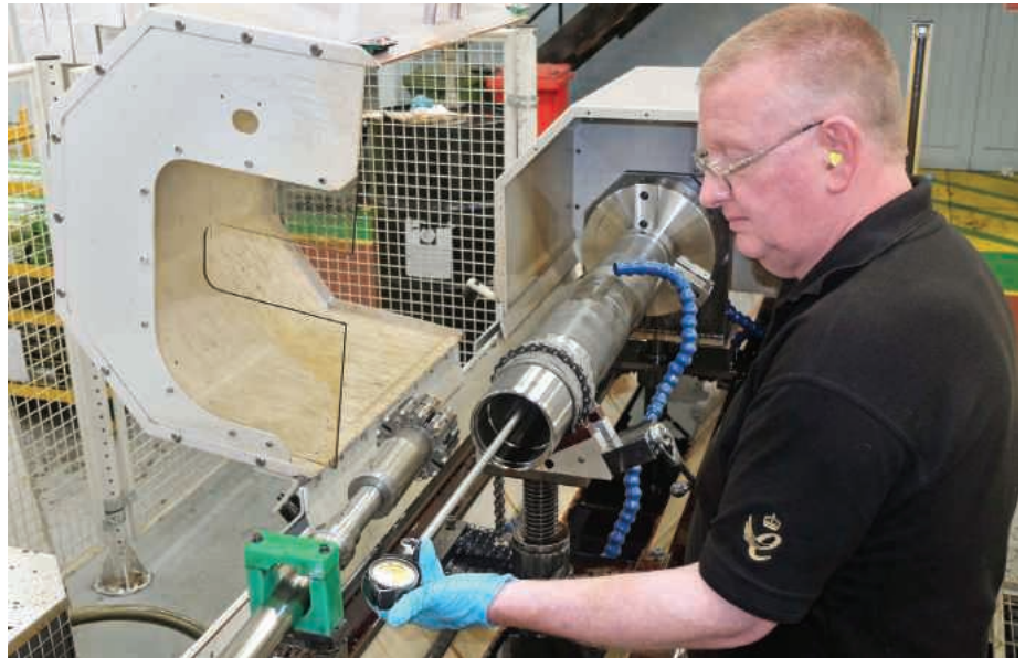
An Oleo Type 70 industrial buffer cylinder secured for horizontal honing on a Sunnen CNC machine. The chain clamp at one end, which is supplied with the machine, would be insufficient to hold the part firmly enough, hence the use of a Kitagawa JN12T manual scroll chuck at the far end
