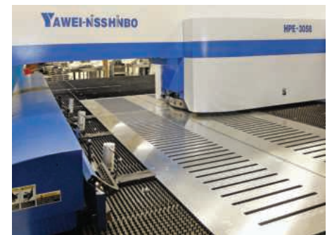
A view from either end of the punch press showing 3 mm thick aluminium sheet being machined for new student residential accommodation at Eastside Locks in Birmingham
