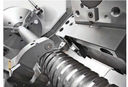
A 40 mm diameter, 2.5 metre long steel ballscrew being machined on an NZX 4000 in a cycle time of 14 minutes 10 seconds
