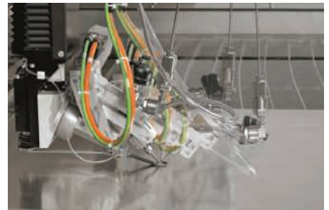
The cutting head revolves only around the focal point of the cutting nozzle. This enables a precise cutting process
