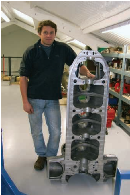
This 1.4 M long cylinder block casting was machined on the Bridgeport GX 1600
