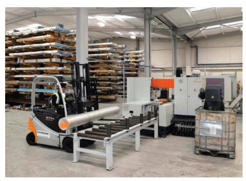
280 mm diameter aluminium bar being delivered by fork lift truck to the KASTOtec AC4 bandsaw at the new Metalex branch in Birmingham
