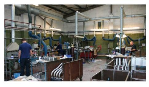
growth and diversification, part of the Iracroft investment has been used to expand the tube manipulation, fabrication, orbital welding and oil pressure testing departments. In these departments, Nederman has been instrumental in delivering a clean working environment.
