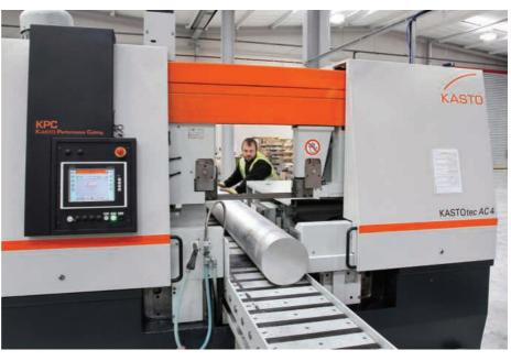
A roller infeed conveyor assists movement of the stock into position
