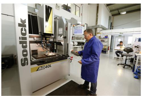
The AG40L EDM incorporates a number of innovative features, including Sodick linear motors, which have a 10 year positioning accuracy guarantee, the latest no-flush EDM technology and energy saving circuits, zero electrode wear, and increased machining speeds. The XYZ travels are 400 x
