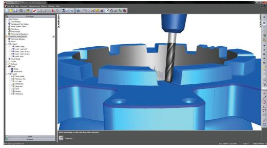
of improvements. These include support for different types of roughing links, wind-fan approach and retract moves for finishing, better gouge checking for plunges and retracts, and tool radius and partline cutter compensation support.
