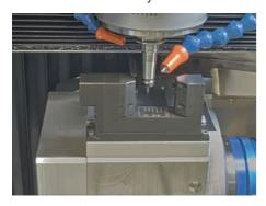
directly in the working space, ideally immediately adjacent to the tool holder. "This enables all influences, such as temperature-related expansion of the machine, to be measured and taken into account. The thermal expansion of the spindle and the tool fitting, as well as the speed-related displacement of the spindle, can also be compensated, which is essential when accuracy levels of less than ten microns are required."
