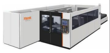
Steve looked at a number of different machines but eventually settled on a Mazak OPTIPLEX 3015 II which is equipped with a high power 4 kW resonator and is capable of 120 m/min rapid traverse rate delivering ultra-high speed cutting times and exceptional accuracy. What swung the decision was the aftersales service that Mazak was prepared to put in place.
