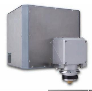
placed great emphasis on industrial suitability. The system has modular construction and active water cooling. Its sealed, gas-purged beam path always ensures cleanliness. This makes precSYS a low-maintenance product with resilience against fluctuating temperatures, ablation particles, dust etc. It is very precisely factory-pre-calibrated and can be equipped with optional automatic fine alignment. The system offers two observation ports for process-monitoring add-ons.
