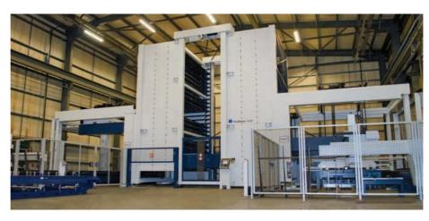
Using BrightLine fiber, it's possible to switch from thin to thick sheet processing on a single machine platform without any loss of quality. Up to 25 mm thick steel, stainless steel and aluminium can be cut using a solid state laser with excellent edge quality. In short, BrightLine fiber is a technology that enables vast beam diameter adjustability, a capability that conventional fibre lasers lack.
