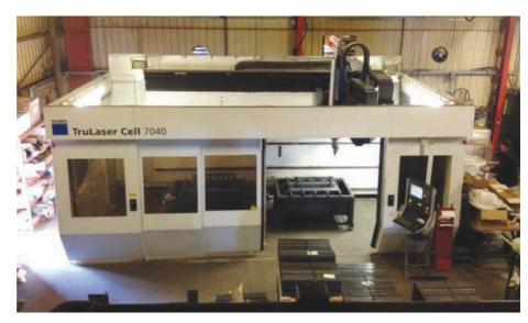
In addition to the fibre laser, the company also installed a new TRUMPF 7040 twin cab 5-axis laser cutting machine in February to replace its previous 5-axis machine. The machines are used to provide three-dimensional cutting of parts that have already been deep-drawn, formed or manipulated.
