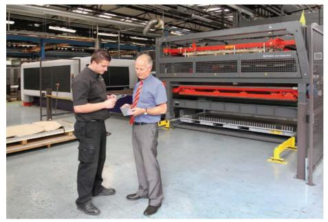
The sides, roof and doors of welfare units manufactured by Groundhog (UK) are made from 1.5 mm thick sheets that are cut three times faster on the new Bystronic fibre laser compared with the former CO2 laser machine
