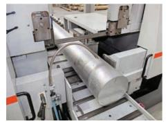
The bar in position, ready to be clamped for cutting
