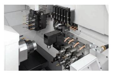
The three new versions all feature new wider access to the working zone through a rising and hinged operator door plus additional rear access. Main and sub-spindles have 7.5 kW and 3.7 kW motors respectively, providing 8,000 revs/min and driven tool speeds of 6,000 revs/min from 1 kW motors.
