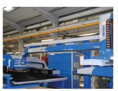
E5 punching machine with LST automation
