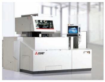
The MV2400-SZ+ also features a new, non-contact cylindrical drive system and the M700 series control with a particularly large 15-inch touch-screen. This Windows based control is both intuitive and user friendly and with the 15 inch screen, it improves operation for the end user.
