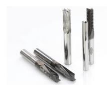
machining of special fibre-reinforced thermoplastics, predominantly carbon fibres. As carbon fibres are very abrasive, the solid carbide milling cutter is diamond coated. Thanks to the arrangement of the cutting edges around the circumference, the fibres are cut off cleanly without burn
