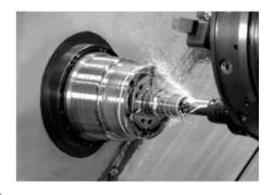
tools. Additional benefits of the TOPlus include the elimination of radial displacement between clamping head and chuck body, which makes it resistant to contamination. Furthermore, the chuck incorporates vibration damping technology that also enables the end user to improve surface finishes and precision levels.
