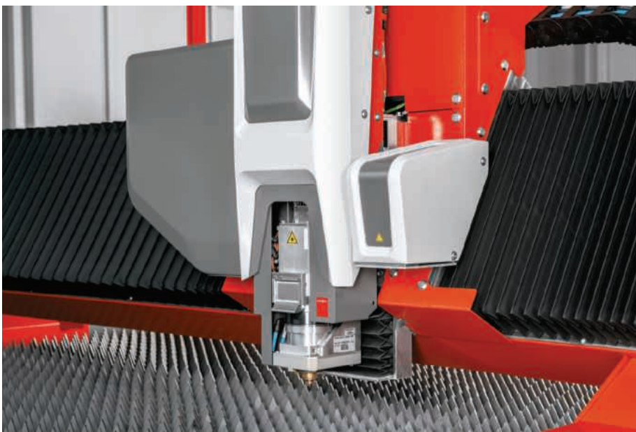
Speed and consistent quality: The new cutting head adapts the laser beam with high precision, depending on the material and sheet thickness
