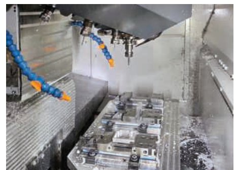
The machining area of the R650X1, showing the use of multiple fixtures so that one part comes off the machine complete per pallet change
