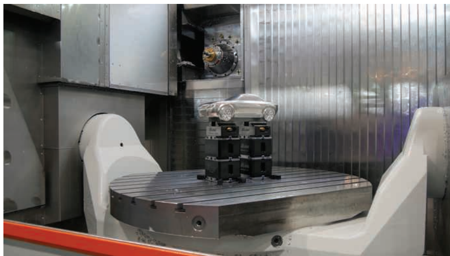
The 5-axis PBZ HD profile machining centre provides heavy duty machining for workpieces up to maximum 30,000 mm in length
