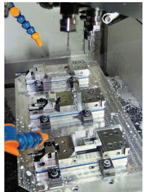
The machining area of the R650X1, showing the use of multiple fixtures so that one part comes off the machine complete per pallet change
