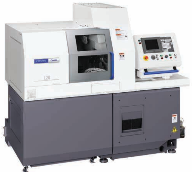
The Citizen L20-VIII used to demonstrate LFV high technology cutting
