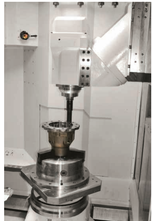
With the NC swivel head providing five-axis machining capability, and a rotary table option offering turn-mill operations, the HEC630D U5 MT is the latest addition to Heckert's large-capacity machining centre range.
