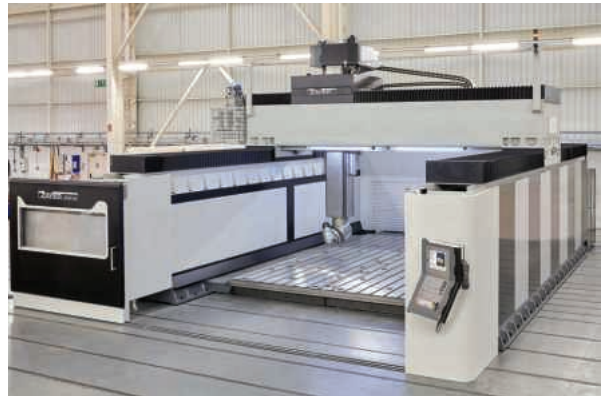
The MEMPHIS 7000 high speed, 5-axis machining centre pictured at the Zayer factory before being shipped to Batz
