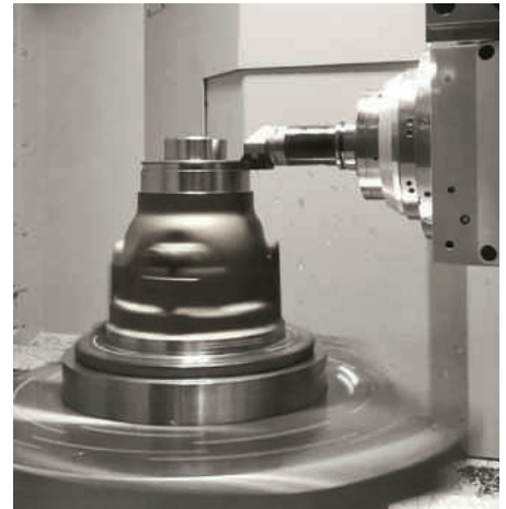
With the NC swivel head providing five-axis machining capability, and a rotary table option offering turn-mill operations, the HEC630D U5 MT is the latest addition to Heckert's large-capacity machining centre range.
