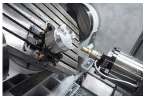
A view of the uprated 83 kW spindle on the HEC 500 X5
