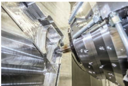
The new 150 kW spindle version on the Scharmann Ecospeed F
