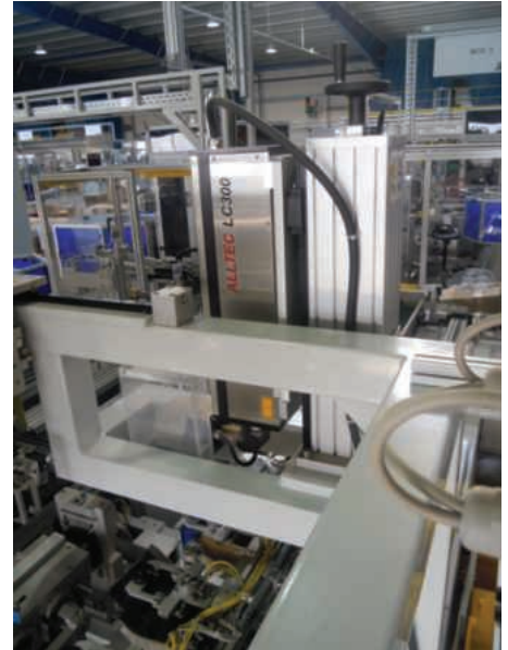
Just one of the six FOBA laser marking systems used by Raval at their Luxembourg manufacturing site
