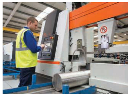
The second KASTO bandsaw installed by Langley Alloys is a purpose-built 'carbide' version, KPC, which has additional equipment designed to suppress vibration
