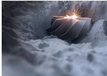
With the powder bed technique very small, highly complex filigree parts can be manufactured by means of selective laser melting
