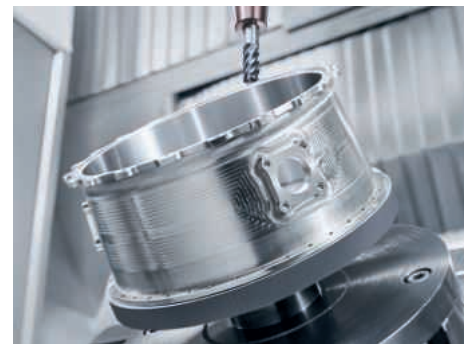
The powder nozzle and milling head of the LASERTEC 65 3D hybrid can be changed at any time, so that areas of complex geometries can be milled that would no longer be accessible subsequently on the finished part
