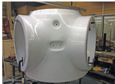
MHP also produce other items using Vacuum Forming programmed by Tebis including hubs for wind turbines and parts for full size motorcycle kits
