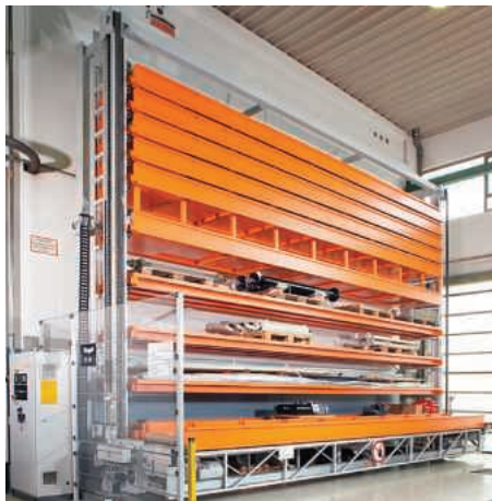
The KASTOunitower tower storage system is a space-saving, economical alternative to floor and cantilever arm storage systems
