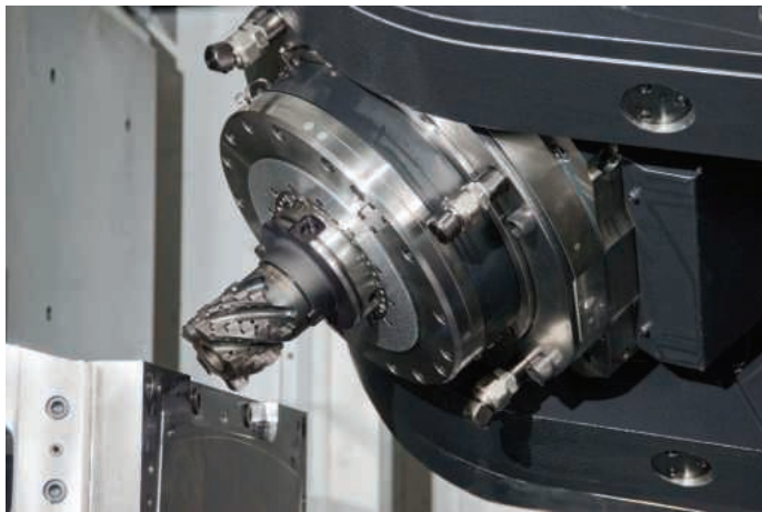
Makino's ADVANTiGE titanium machining takes advantage of an HSK-A125 / 4,000 rpm or 8,000 rpm integral drive spindle with 150 kW of power and 1,500 Nm of duty rated torque (1,000 Nm continuous)
