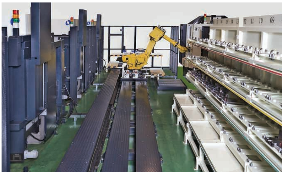
A fixture plate being selected by robot from the storage racking of an MMC-R system
