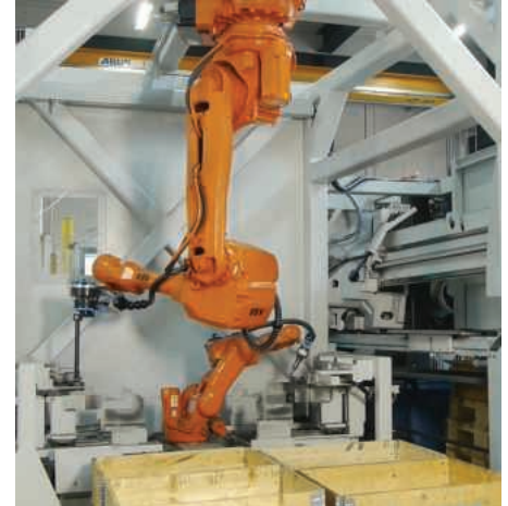
With the KASTOsort robotic sorting system, cut pieces can be stacked, deburred, cleaned, weighed and marked automatically
