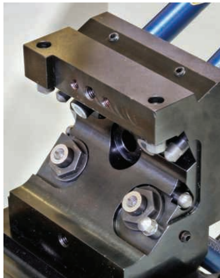
Close-up of the fixture with the test blade removed, showing the four grippers before application of Blue Photon adhesive. The UV light guides may be seen top and bottom right
