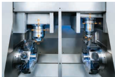
The two work areas of the VL 3 DUO are each equipped with a 12-position tool turret
