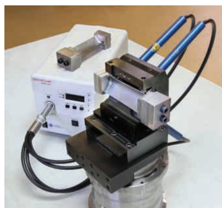
The fixture designed by NCMT for securing a turbine blade on one aerofoil surface using four adhesive grippers so that the root and shroud features can be VIPER-ground in a single cycle
