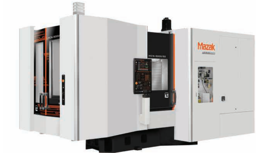
The HCN 5000/50 is a new 50 taper machine with a 500 mm square pallet boasting extremely agile performance characteristics, including a 10,000 rpm/ 37 kW high performance spindle; rapid traverse rates of 60 m/min in the X, Y and Z axes and a chip-to-chip change time of only 3.5 seconds
